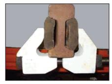
Bull Head Clamp for Ballasted Track 2 per joint Req. Torque setting 220-240 ft lbs / 300-325 Nm Deep Socket Required Stores No. 610/9759A
